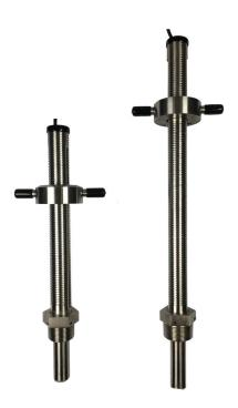
The Signet 2552 Metal Magmeter from Georg Fischer features all-stainless steel construction. The PVDF nosepiece and FKM O-rings are the only other wetted materials. The 2552 installs quickly into standard 11/4 in. or 11/2 in. pipe outlets, and is adjustable to fit pipes from DN50 to DN2550 (2 to 102 in.). Two sensor lengths allow maximum flexibility to accommodate a variety of hardware configurations, including ball valves for hot-tap installations.
