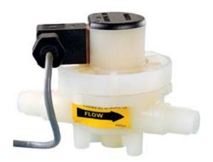
The Signet 2507 Mini Flow Rotor Sensor contains a free-running rotor that is driven by the fluid flow. Within the given measurement range, the rotational speed of the rotor is proportional to the fluid flow rate.
